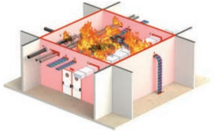
Fire stopping products are used to contain fire and restore the fire rating of walls and floors.
