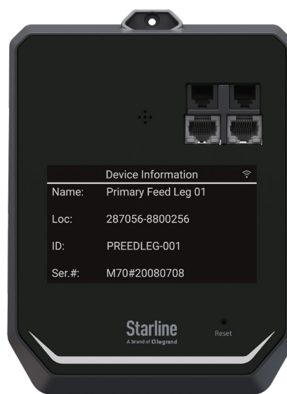
M76 Wi-Fi + (2) RJ11, (2)RJ54, Lg. Display
